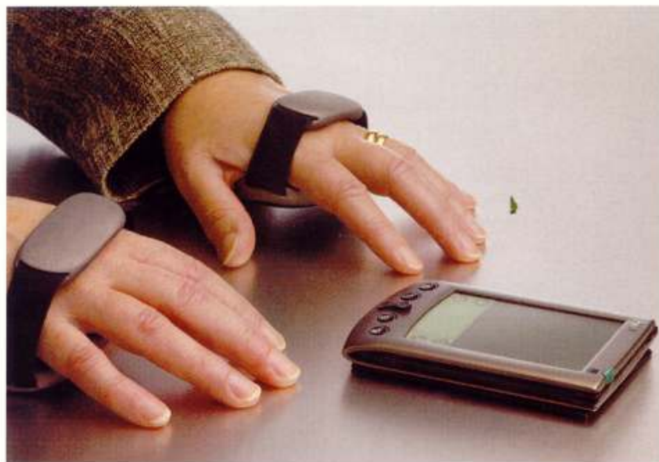
Senseboard's Virtual Keyboard uses sensors to detect the keys you would be typing on a real keyboard.
